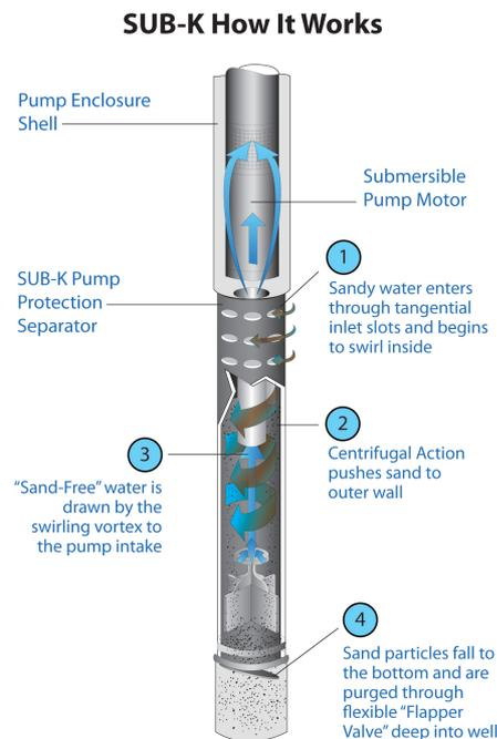
**Figure 10. A cutaway diagram of a down-hole separator.**
