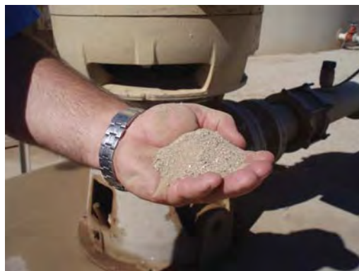
(Pictured Above) Ron Baysinger of Queen Creek Water Company next to one of nine LAKOS protected turbine pumps. (At Left) Damaging sand found in high flow wells in the central Arizona area
