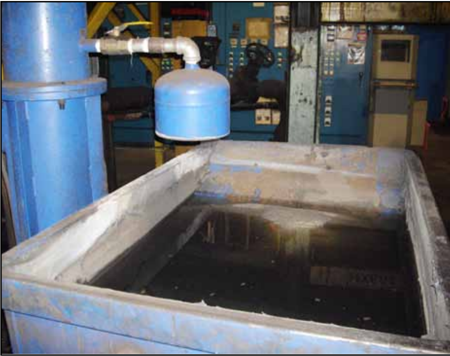
The LAKOS Separator purges into a special hopper that allows for water to rise and overflow going back to the original tank. This allows for the removal of only the scale, which sinks in the tank.
