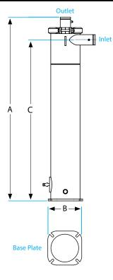
Recommended direction of inlet/outlet piping to control vibration
