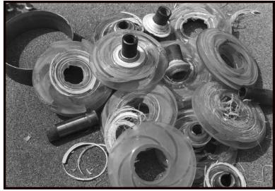
These "remains" of Brewer's second pump are clear evidence of what sand does to a pump's impellers. Lost efficiency, increased power usage, pulling the pump and replacing the damaged parts are costs he can now control with a LAKOS Pump Protection Separator.
