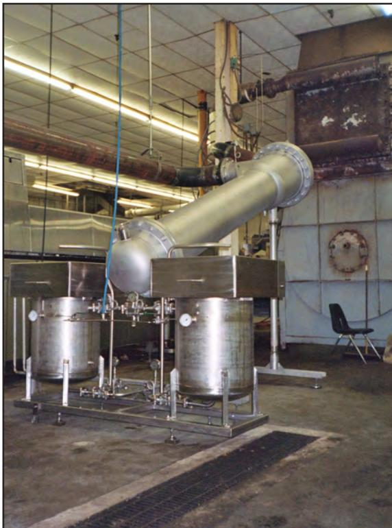
*FrySafe System showing purge and heat exchanger in the background.*
