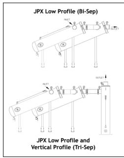
Multiple separators in series - example configurations
