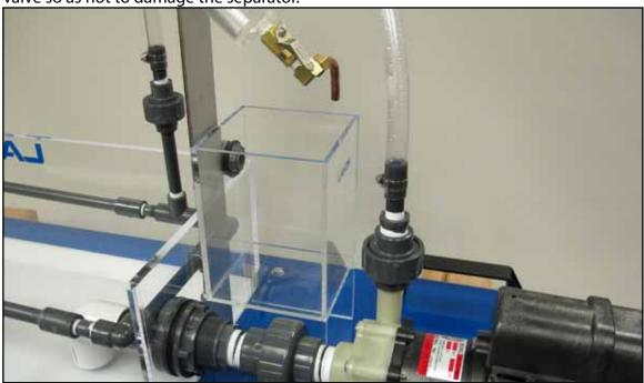
9. If hopper is not to be used, use the small piece of included hose to purge the separator directly into the basin.
