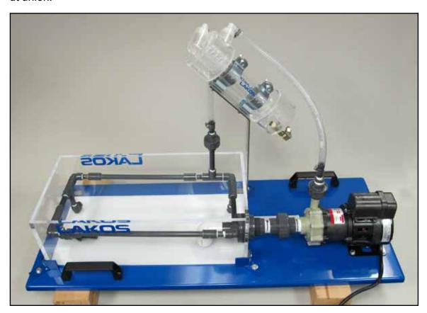
7. Place hopper on skid under separator so that overflow empties into tank.
