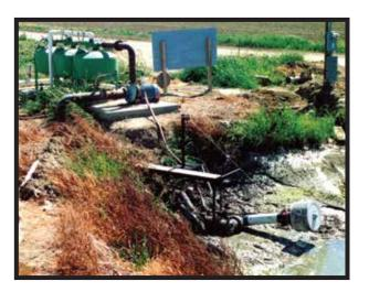
PC Screens protect pumps and water systems from source water organics and debris. They provide a continuous defense against clogging, lost suction, and pump wear.
