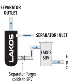
Solids Recovery Vessel (SRV) helps capture separated solids from LAKOS Separators – and return clean liquid back to the system through pump suction for zero liquid loss
