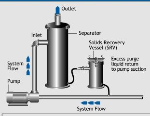
LAKOS Separators & Systems must be installed downstream of the main System Pump. Do not install on the suction side of the main system pump. Flow must be pushed through the separator and not pulled. Consult LAKOS for questions.
