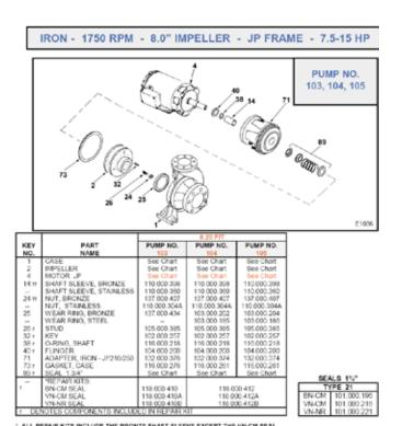
ALL REPAIR KITS INCLUDE THE BRONZE SHAFT SLEEVE EXCEPT THE VN-CM SEAL, WHICH IS STAINLESS.
