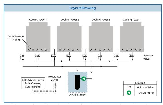
1. All wiring, conduit, and fittings from the control panel to the actuator/valve assemblies to be sized and provided by others. 2. Multi-Tower Basin Cleaning control panel is powered separately from the LAKOS Filtration system.
