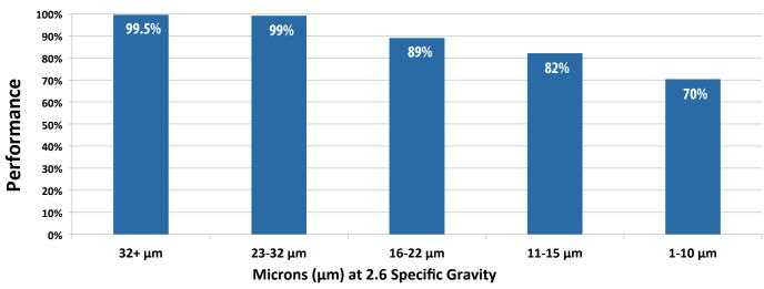
The above efficiency results were based upon 20% side stream within 16 hours. Field results may vary depending on side stream percentage and basin size.
