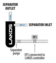
EFS and LAKOS Controller automatically purge separated solids from Separator's collection chamber at pre-determined time intervals — eliminating manual purging.
