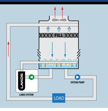
Traditional side stream filtration systems take a percentage of the flow (generally 10-25% or less) from the main line using a by-pass directly to the filtration system. The filtered water is then returned to the main line. Basin sweeping is simply relocating the traditional side stream filtration system from the main line directly to the cooling tower basin, thus increasing the percentage of side stream filtration to 20% or more.
