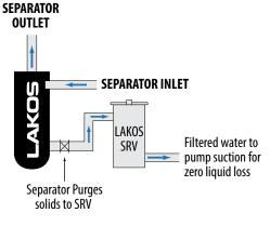
Solids Recovery Vessel (SRV) helps capture separated solids from LAKOS Separators – and return clean liquid back to the system through pump suction for zero liquid loss
