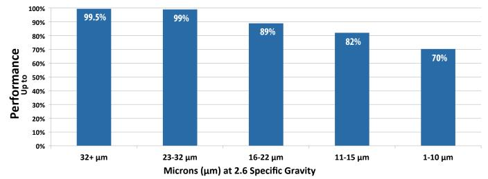
The above efficiency results were based upon 20% side stream within 16 hours. Field results may vary depending on side stream percentage and basin size. Single Pass Separator Performance results verified by Independent Testing.
