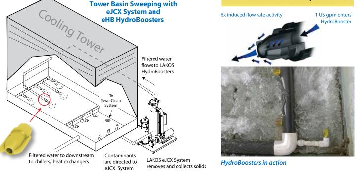
Directed turbulence maximizes cleaning efficiency in the tower basin/remote sump. LAKOS eHB HydroBoosters provide that turbulence with patented vortexing action. Consult LAKOS for technical assistance in basin sweeping layout and piping options.
