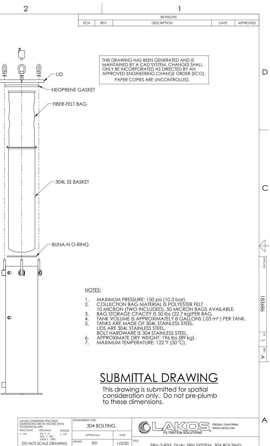
1/3/20 SRV-2-833, DUAL SRV SYSTEM, 304 BOLTING -8" DIA x 33" BAG 3/4" INLET 3/4" OUTLET, SS SIZE MODEL NO. -DWG NO. 183686
