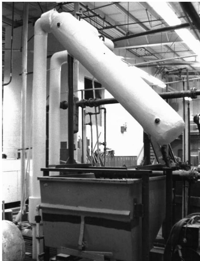
*Above, a Lakos 6" Industrial Separator is installed directly over a solids collection dumpster and, on a continuous controlled flow purge (shown at left), empties the separated solids into the dumpster for eventual disposal.*
