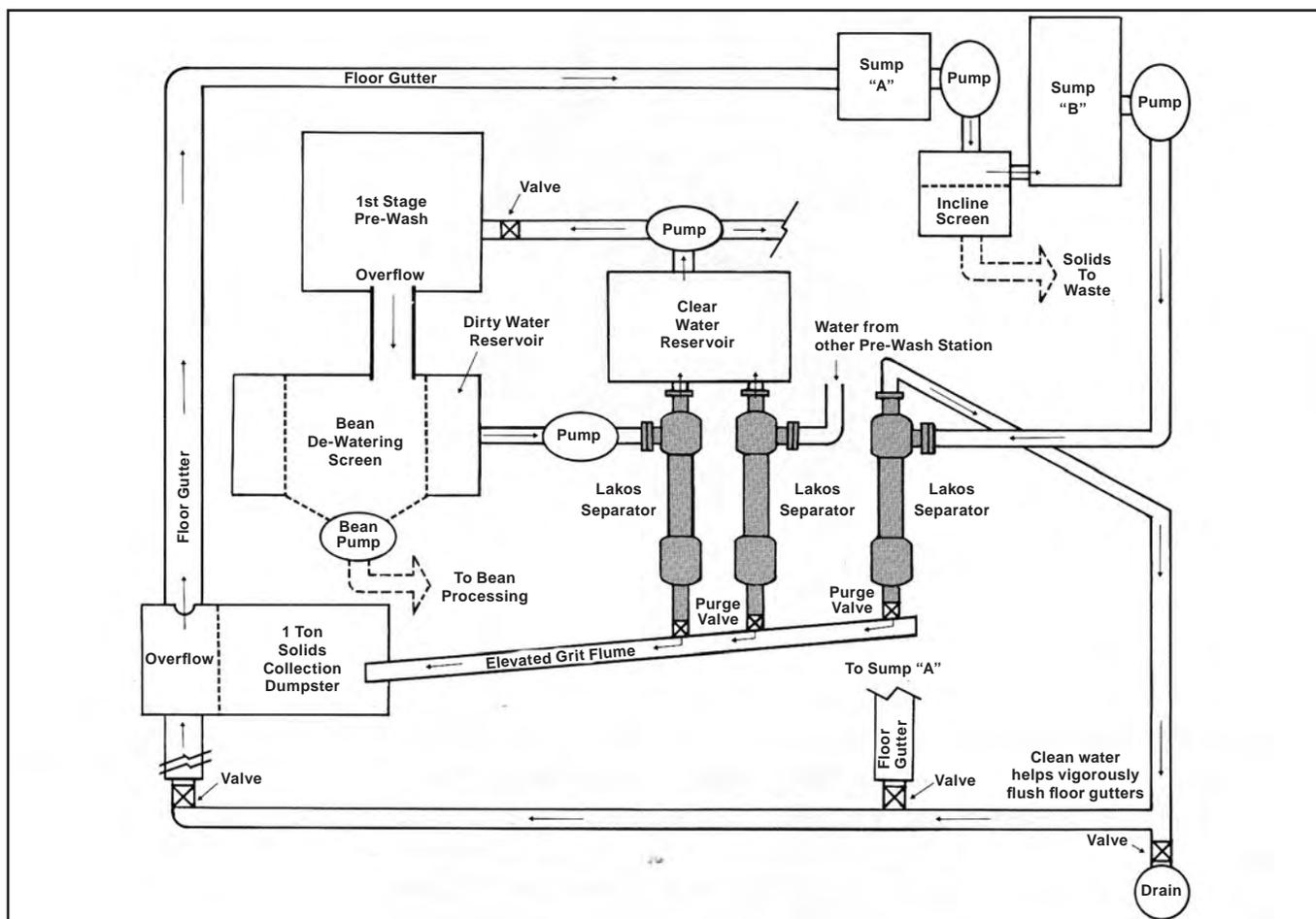
Having already experienced the performance of LAKOS Separators on one of their carrot washing operations, Gerawan implemented a means to continuously and completely recycle the bean washing water through three LAKOS Separators, capable of handling a peak flow demand of up to 1,100 U.S. gpm (250 m<sup>3</sup>/hr.).
