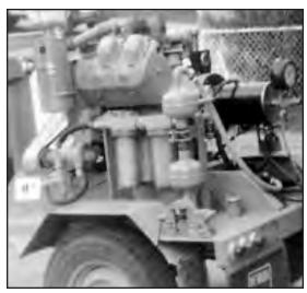
The compact Lakos Separator (see photo) was easily retrofit on Miller's portable hydroblaster system as a pre-filter to the cartridges (see illustration).
