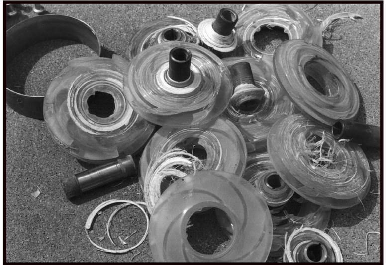
*These "remains" of Brewer's second pump are clear evidence of what sand does to a pump's impellers. Lost efficiency, increased power usage, pulling the pump and replacing the damaged parts are costs he can now control with a LAKOS Pump Protection Separator.*
