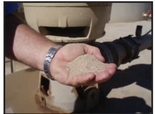
Damaging sand found in high flow wells in the central Arizona area.
