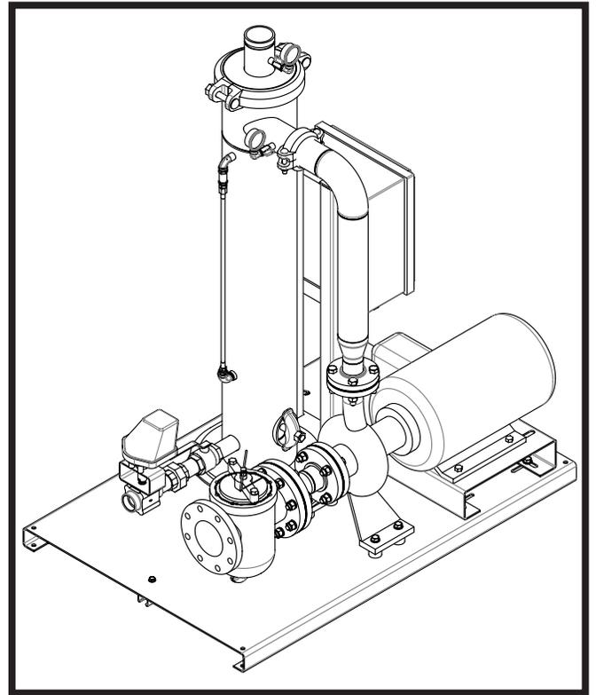
Diagram of a typical JCX tank cleaning package
