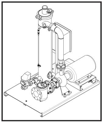
Diagram of a typical JCX tank cleaning package
