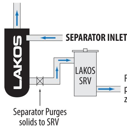
Solids Recovery Vessel (SRV) helps capture separated solids from LAKOS Separators – and return clean liquid back to the system through pump suction for zero liquid loss
