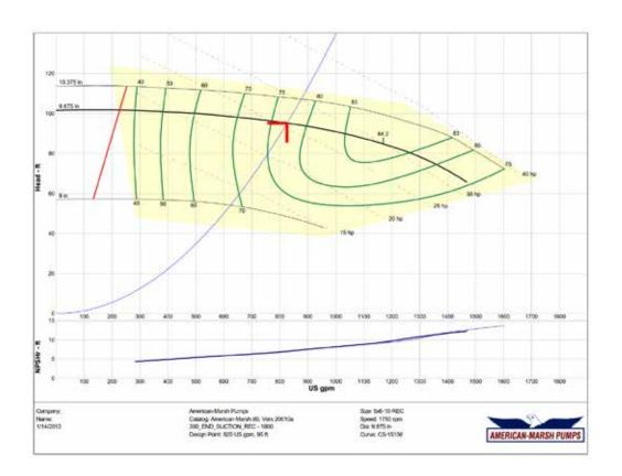
Models: TCX & TCI (1100) Flow-rate: 1100gpm Impeller Trim: 10.38
