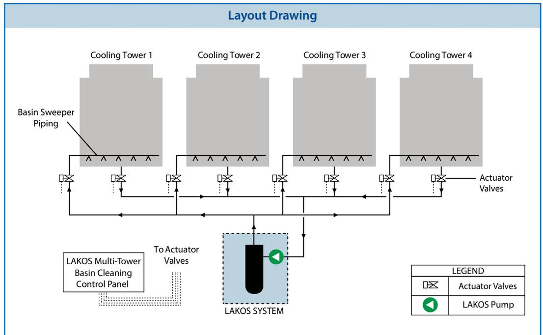
1. All wiring, conduit, and fittings from the control panel to the actuator/valve assemblies to be sized and provided by others. 2. Multi-Tower Basin Cleaning control panel is powered separately from the LAKOS Filtration system.
