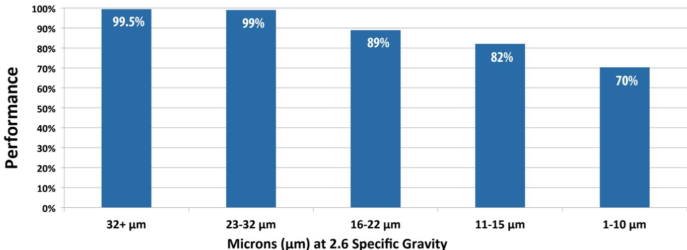
The above efficiency results were based upon 20% side stream within 16 hours. Field results may vary depending on side stream percentage and basin size. Performance results verified by independent testing.
