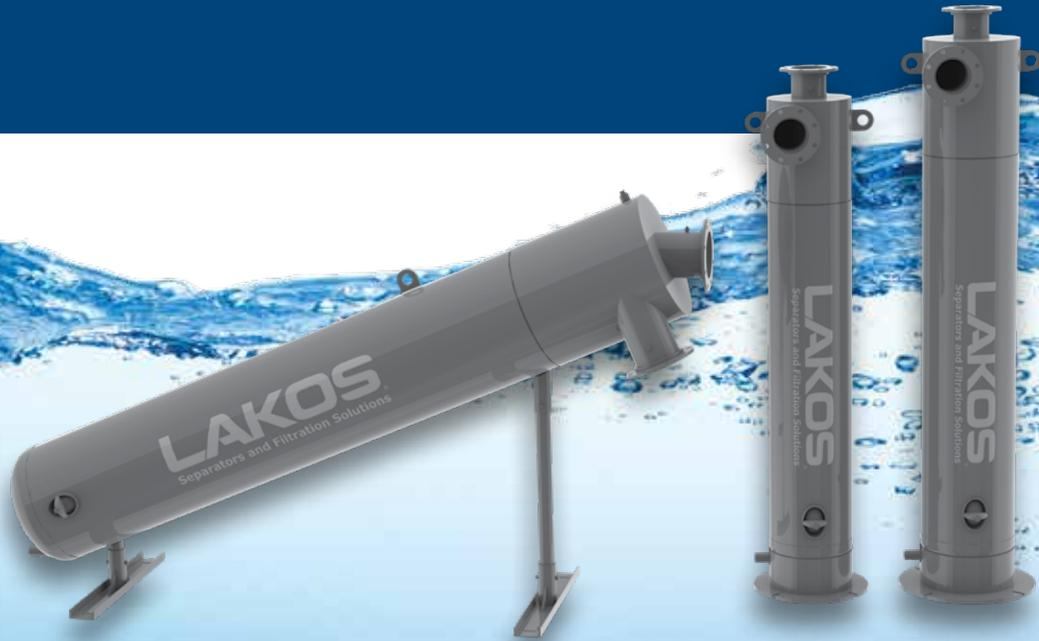
**LAKOS Sand Separators** employ centrifugal-action to remove settleable particles (200 mesh/74 micron sand & larger) from pumped water. With an automatic purge valve, the system is free of routine maintenance. Options for solids removal are also available. NSF/ANSI standard 61 and Annex G
