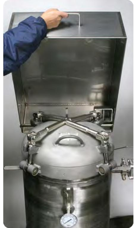
Two manual isolation ball valves, one on the inlet to the collection vessel and one on the discharge or return of the collection vessel, to completely shut-off the flow of oil to the vessel. One set of valves on each vessel.
