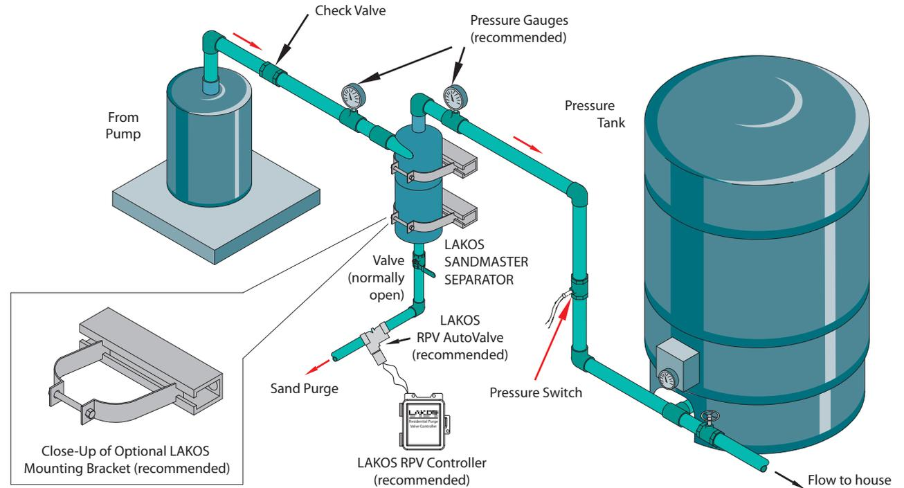
IMPORTANT: Install SandMaster between the check valve and pressure tank.
