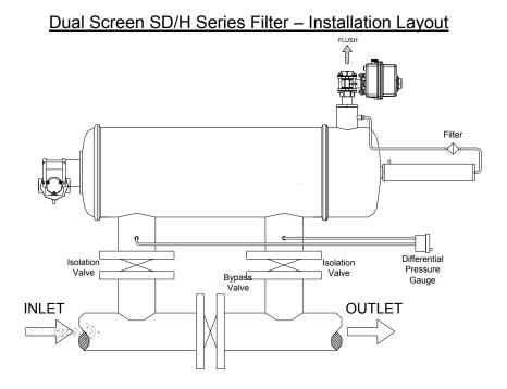
There should be adequate clearance around the filter to allow for easy maintenance access, including a minimum of 24" from the back (piston side). The minimum clearance on the front (cover) depends on the model. There must be enough room to remove the coarse screen and fine screen periodically.
