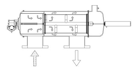
This drop in outlet pressure is monitored by the differential pressure gauge, which at seven PSID (pounds per square inch differential) sends a signal to the controller to initiate a backwash cycle.
