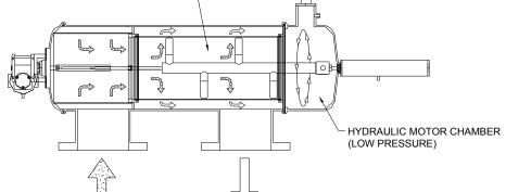
Water flows through the suction nozzles, down the interior of the particle remover, and out the hydraulic motor. The motor rotates the particle remover, enabling each suction nozzle to cover a radial strip of screen. The pressure difference between the interior of the filter and the hydraulic motor chamber drives the particle remover toward the hydraulic piston.
